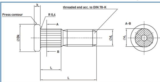
Compared to similar round-bodied press-in fasteners, the TRILOBULAR® shape guarantees a lower press-in force with less variation during assembly. The component's material can flow between the lobes to develop a form-lock between the fastener and the component. In addition, material flow between the knurls provides additional turning resistance.
