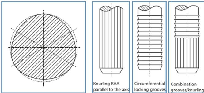
By using TriPress® fasteners, assembly times can be reduced up to 75%. There are no resulting assembly problems, such as cross-threading, which typically occurs with metric screws. The simple TriPress® press-in process, ideally achieved by using displacement-controlled presses, requires less costly assembly equipment and tools.
