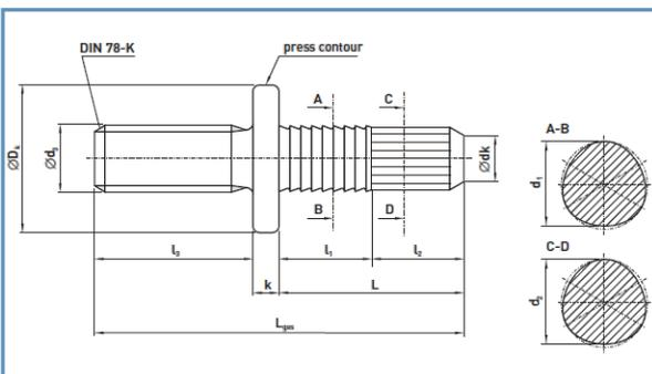
If the primary objective of the assembly process is reduced assembly time, but the application additionally requires good serviceability, we would alternatively recommend our PUSHTITE® II™ fastener design. Similar to the TriPress® fastener, the PUSHTITE® II™ assembly process is accomplished by a simple press-in operation.
