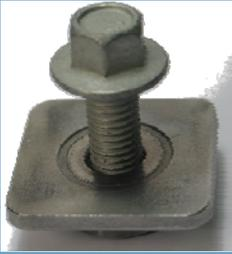
*Figure 1 - Pierce-and-Clinch Nut assembled in HSLA thin-sheet steel*
