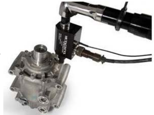
Aluminum Die Cast AC Compressor Being Tested Using Ultrasonic Torque Tension Transducer
