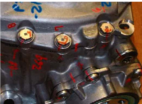
4-Wheel Drive Power Transfer Unit Ready for Ultrasonic Testing
