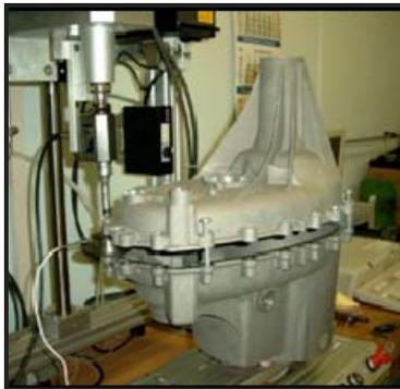
The thread forming torque performance depends on the strength of the nut, the pilot hole diameter, the component thickness (thread engagement depth) and friction relationships. Generally speaking, little can be changed to
