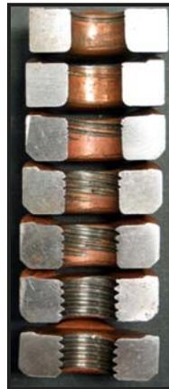
Compared to other thread rolling screws for metal available in the market, the TAPTITE 2000® screw has a patented thread geometry that has been optimized for the material forming process. The
