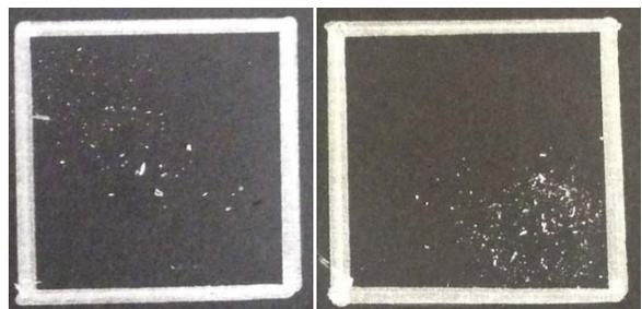
When the screws were thread forming into the AISi9MgMn T5 aluminum, the debris generated was gathered on black paper and placed in a 25mm square. This made it easier to visually compare the amount of debris generated by each screw.
