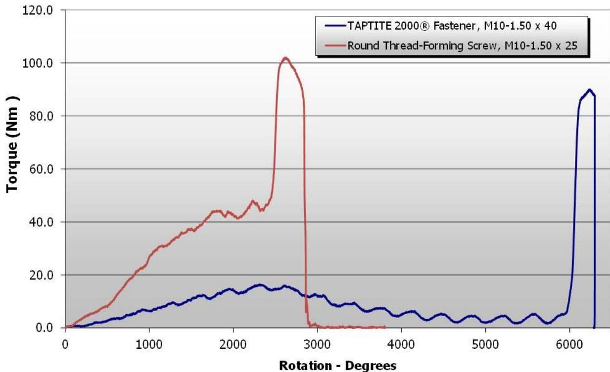
The round thread forming screw required an average thread forming torque (46.2 Nm) that was nearly 3 times higher than the thread forming torque (16.9 Nm) required for TAPTITE 2000® screws.
