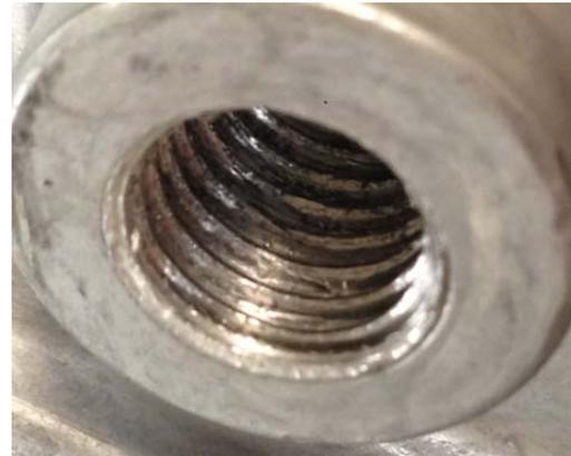
The AlSi9MgMn T5 aluminum reacts to thread forming similar to magnesium. The material does not allow volumetric displacement to occur when forming the internal thread, thus forming a rough internal thread and creating debris, some of which appears to remain lodged in the internal threads.
