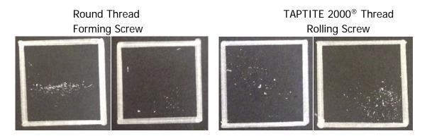
When the screws were thread forming into the AlSi9MgMn T5 aluminum, the debris generated was gathered on black paper and placed in a 25mm square. This made it easier to visually compare the amount of debris generated by each screw.
