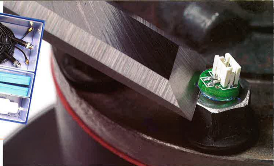
Patented sensor design allows for convenient removal and reuse.
