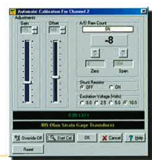
Calibration screen for standard strain gage
